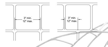
The spacing between the welds should be a minimum of 3" (76mm) apart and a maximum of 12" (305mm) apart. When welds are closer or spanning farther than
