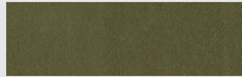
SR Evergreen (SRI = 33) Reflectance: .32 Emittance: .88
